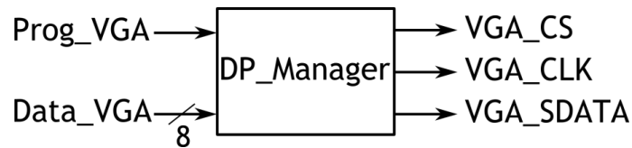
Figure 3.23 Block diagram of the amplifying gain control unit.
